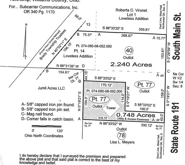
All dimensions are shown in feet and decimal parts thereof. This survey has been recorded in Volume Page, of the Williams County Record of Surveys. 10V 263
